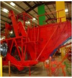
Built in 1920, the Harris Combine has a four cylinder gas engine, 55 horsepower, and a 24 foot header. It took 5 people to operate: 2 sack sowers, a header tender, a separator attendant and a tractor driver. This Harris harvester would average 1200 to 1300 sacks per day or 60 to 65 tons.
